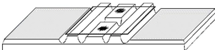
There are four longitudinal grooves in the central third of a rectangular and thick base plate made of special optical glass.
